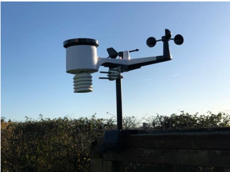
Figure 12.18: B-Fluid On-site Weather Station
