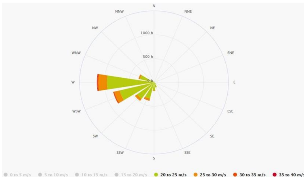
Figure 12.121: Hourly Dublin Wind Gust Rose - Cumulative hours when the velocity is above 20 m/s.
